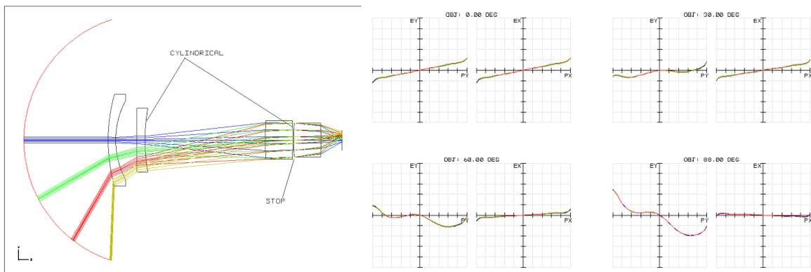
Figure 4 Starting configuration, 4 lenses, all germanium (ray fan scale is 200  $\mu\text{m}$ )
