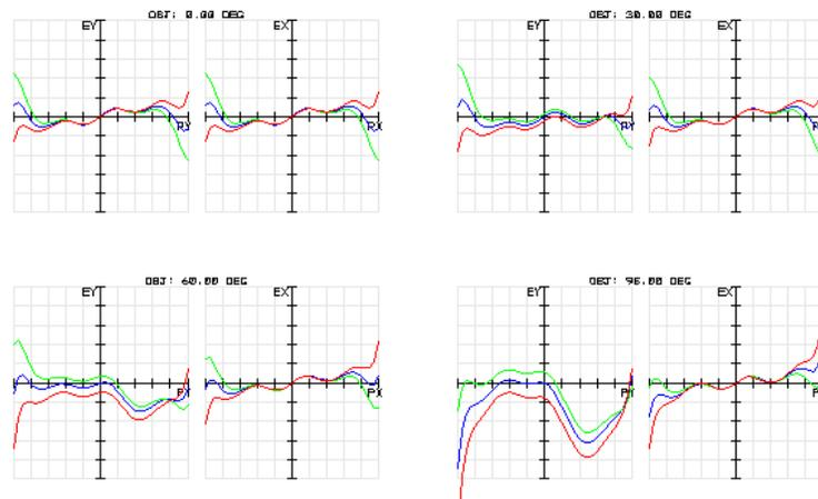
Figure 6: Ray aberration curves for the long axis (scale 20  $\mu\text{m}$ )
