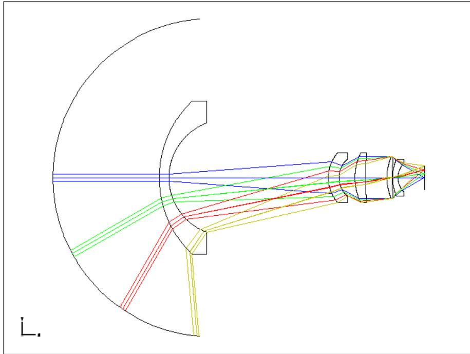
Figure 5: First design layout (lenses 2 and 4 are cylindrical, lenses 1 and 5 are aspheric)
