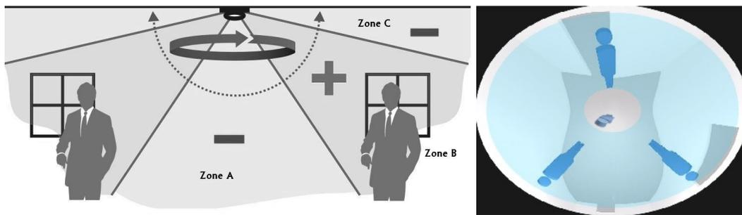
Figure 1: Specific security zones and image footprint on the sensor (elliptical).
