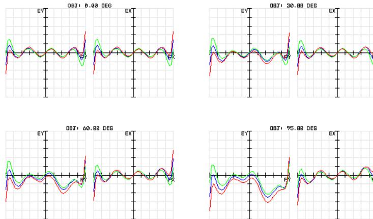
Figure 7: Ray aberration curves for the short axis (scale 20um)
