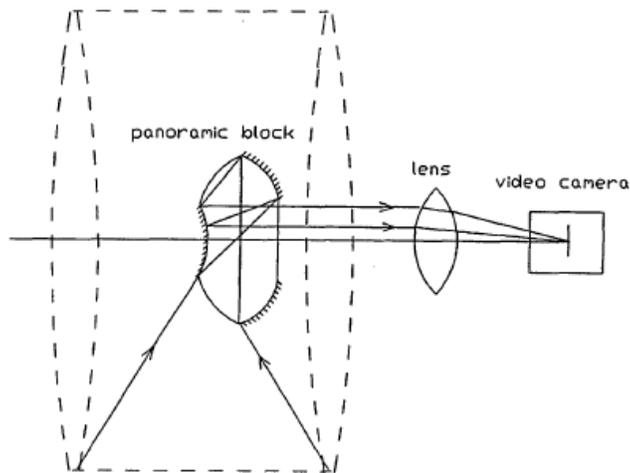
Figure 3: Optical arrangement proposed by Greguss
