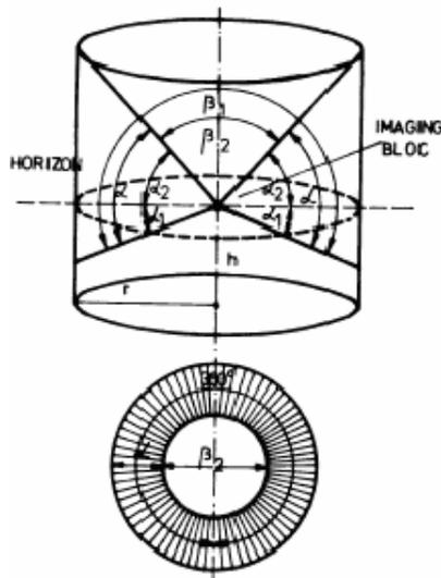
Figure 2: Flat cylinder perspective
