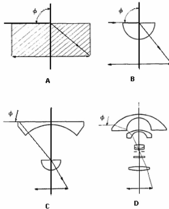
Figure 1 A-D: Development of fisheye lens<sup>2</sup>
