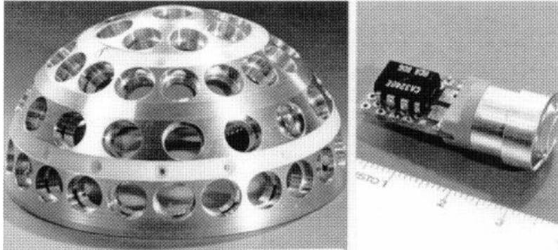
Figure 4: Hemispheric alerting demonstrator, working in the NIR, developed by TNO-FEL
