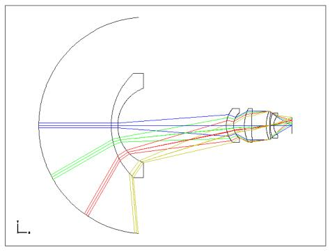
Figure 5: First design layout (lenses 2 and 4 are cylindrical, lenses 1 and 5 are aspheric)
