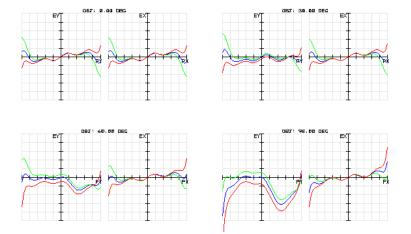
Figure 6: Ray aberration curves for the long axis (scale 20 µm)
