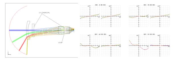
Figure 4 Starting configuration, 4 lenses, all germanium (ray fan scale is 200 µm)
