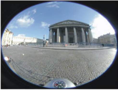
Figure 4. Images taken with a fish-eye lens show improved pixel coverage with an elliptically shaped footprint (top) and a circular one that underutilizes the available pixels on the sensor (bottom).
