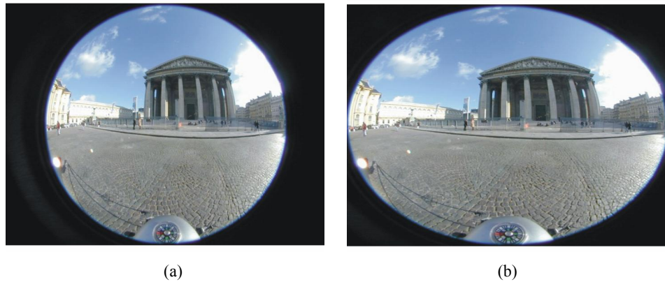
Figure 1(a): Fish-eye lens generates circular image; (b) Anamorphic lens produces elliptical image.
