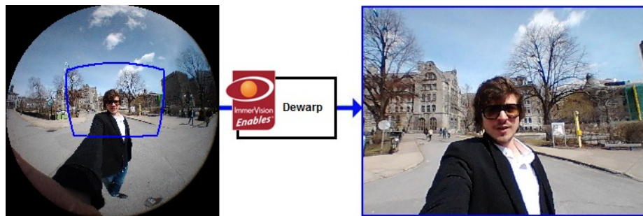
Figure 5: One to one video chat picture captured by the 3.80 mm panomorph lens and one example of a resulting dewarped images.
