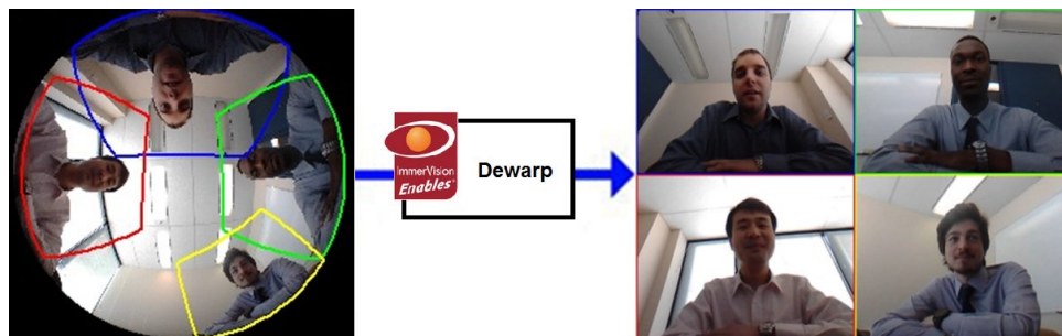
Figure 6: Many to one video-chat picture captured by the 3.80 mm panomorph lens and one example of 4 resulting dewarped images.
