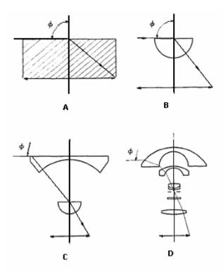
Figure 1 A-D: Development of fisheye lens<sup>2</sup>
