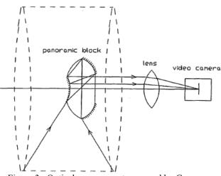
Figure 3: Optical arrangement proposed by Greguss
