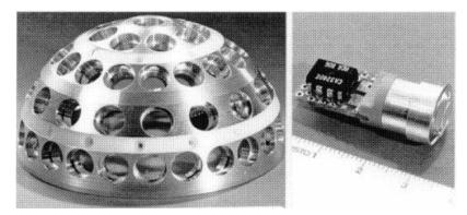
Figure 4: Hemispheric alerting demonstrator, working in the NIR, developed by TNO-FEL
