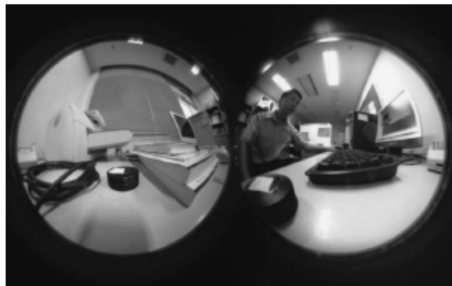
Figure 3 : Full-view spherical image acquired by the spherical image sensor shown in Figure 2 7 .
