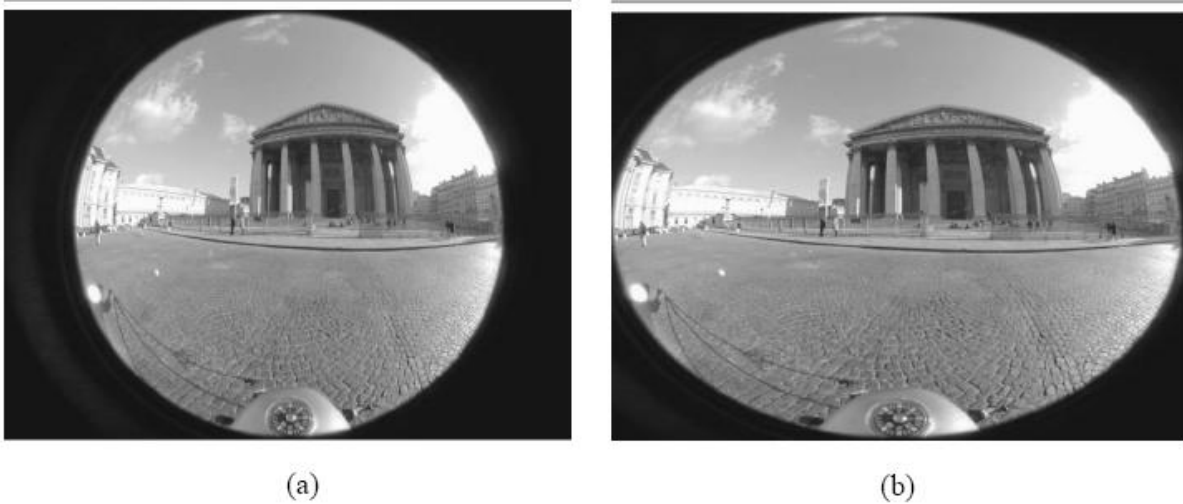
Figure 3(a): Fish-eye lens generates circular image; (b) Anamorphic lens produces elliptical image.
