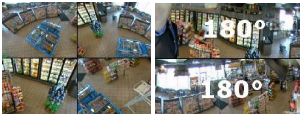
Figure 5: Four PTZ views (left), two strips to display a 360° total camera surround in one single view (right).
