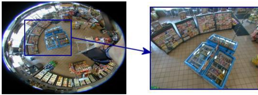
Figure 4: Real-time distortion-free display (left: the original image produce by the panomorph lens).
