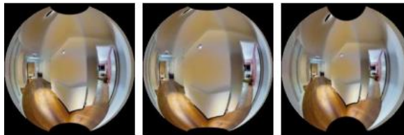
Fig. 1. distortion simulation for each lens model : edges augmented, center augmented, Fisheye
