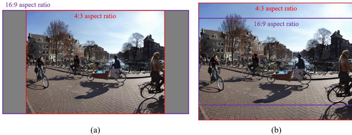
Figure 6. Widescreen image captured on a 4:3 aspect ratio sensor with a rotationally symmetric lens. (a) the black bars are added on the left and right sides to accommodate 16:9 wide screen video format; (b) the top and bottom of the image go unused to accommodate a super wide-angle image 4:3 to 16:9 wide screen movie format.
