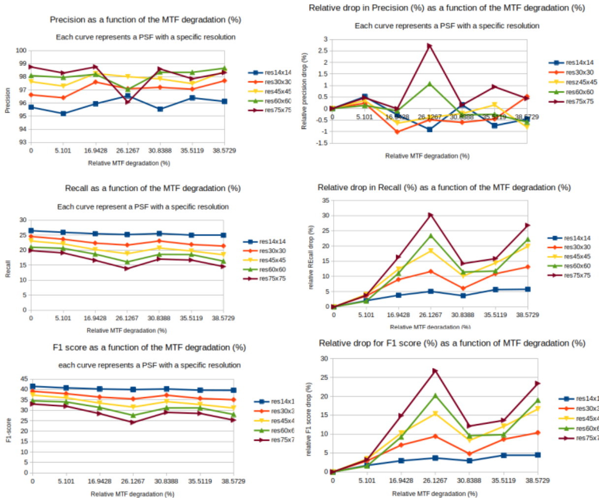
Figure 6. Quantitative results. From top to bottom: Precisions, Recall and F1-score obtained on a subset of PixSet. For each row, the absolute values are presented on the left and the relative drop on the right
